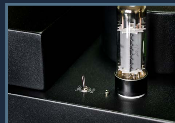
6n2p / 12ax7 and tetrode / pentode mode switches for Luna Prestige
